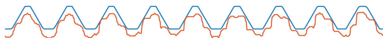
Figure 4-2: Comparison of ideal and measured (photographed) thread silhouette, from Paper 1 in Part 2 of this thesis.
