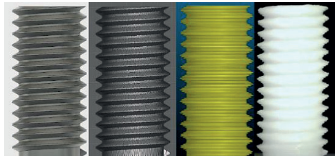
Figure 3-5: Images of the different results from each step in the path from design to physical part using FDM: 1) CAD model, 2) STL file visualization, 3) G-code toolpaths, 4) printed geometry. Image from appended Paper 1.
