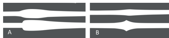
Figure 18: Illustration of experimental width (top) and simulation of flow rate (bottom) results for 0.3 mm layer height, and A) acceleration region for K_{LA} = 0.2 and B) deceleration region for K_{LA} = 0 . Edges traced using the software Inkscape for image clarity.
