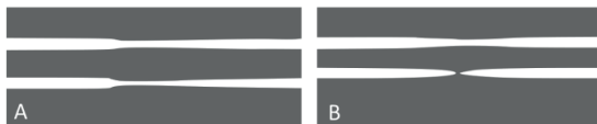
Figure 19: Illustration of experimental (top) width and simulation (bottom) of flow rate from results for 0.3 mm layer height, and A) acceleration region for K_{LA} = 0 and B) deceleration region for K_{LA} = 0.0 . Edges traced using the software Inkscape for image clarity.
