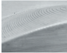
Fig. 4. Layering effect of a printed inclined plane.
