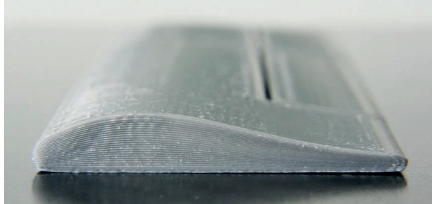
Figure 4-7: Intra-layer variable layer height, limiting the stepped surface, and hence improving the surface finish and dimensional accuracy of an airfoil profile, from Walter [45].
