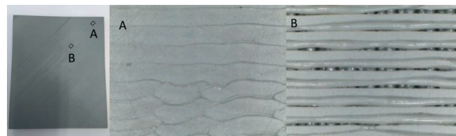
Figure 4 - First-layer-defects due to A) excessive accumulation of material where the nozzle is too close to the print bed, generating a wash-boarding effect, and B) insufficient infill due to too large distance between nozzle and bed.
