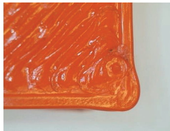
Figure 4-3: Disfigured corner due to inaccuracy during material extrusion, also called corner blob.
