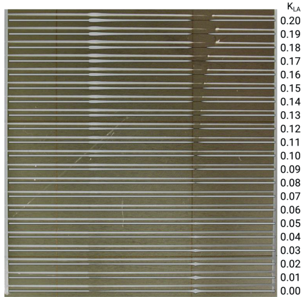
Figure 16: Experimental results for 0.2 mm layer height alongside simulation results for ideal K = 0.06s
