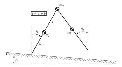
Figure 3.1: Schematic of the planar compass-gait biped on a shallow slope with angle  $\psi$ .
