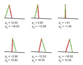
Figure 4.1: Illustration of a complete step of a periodic gait. The values  $q_1, q_2$  are the angles in degrees of the stance leg (red) and swing leg (green) respectively.
