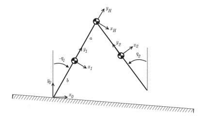
Figure 3.2: Assignment of origins for the coordinate frames of the biped.
