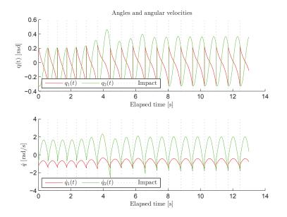
Figure 7.11: Time evolution of q,  $\dot{q}$  for unstable gait at  $\psi=3.00.$
