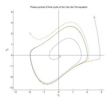
Figure 2.2: Phase portrait of the Van der Pol equation with stable limit cycle, initial conditions are depicted as circles on the three trajectories.
