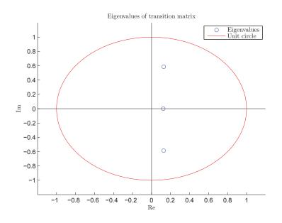
Figure 7.1: Eigenvalues of the transition matrix  $\Xi(x_{\star}^-, x_{\star}^+)$  for the stable periodic gait with  $\psi = 3.00$  degrees.
