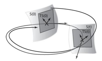
Figure 6.1: Visualization of moving Poincaré surfaces  $S(\cdot)$  and transverse linearization  $TS(\cdot)$  of periodic orbit (grey) and another solution converging to the orbit (black). Illustration © 2008 Elsevier. Reproduced, with permission, from Annual Reviews in Control, vol. 32, no. 2, A. Shiriaev, L. Freidovich, and I. Manchester, "Can we make a robot ballerina perform a pirouette? Orbital stabilization of periodic motions of underactuated mechanical systems," pp. 200 211, 2008.
