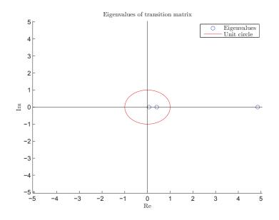
Figure 7.8: Eigenvalues of the transition matrix  $\Xi(x_{\star}^{-}, x_{\star}^{+})$  for the unstable periodic gait with  $\psi = 3.00$  degrees.
