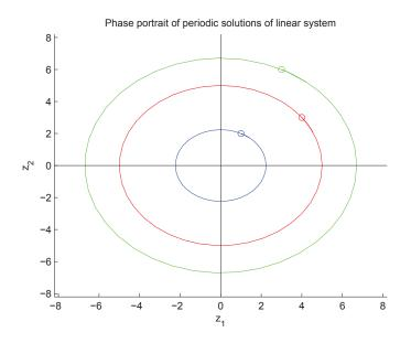
Figure 2.1: Phase portrait of a linear system on the form (2.17), initial conditions are depicted as circles on the closed orbits.
