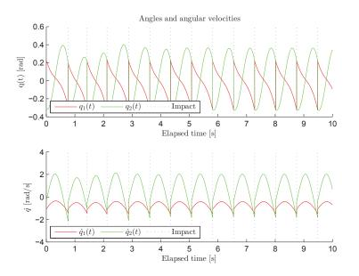
Figure 7.6: Time evolution of  $q, \dot{q}$  for stable gait with perturbation  $\epsilon = [0.01, 0.01]^T$  in initial conditions at  $\psi = 3.00$ .
