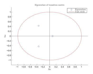
Figure 7.15: Eigenvalues of the transition matrix  $\Xi(x_{\star}^{-}, x_{\star}^{+})$  for asymmetric gait at  $\psi = 5.00$ .
