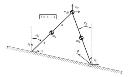
Figure 3.3: Assignment of reference points for impact maps and impact forces.
