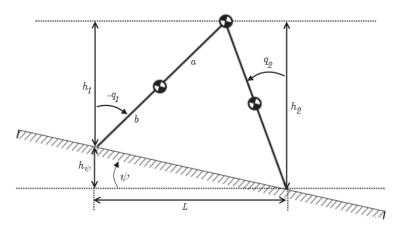
Figure 3.4: Illustration showing the different quantities used when defining the impact surface of the biped.
