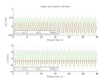
Figure 7.14: Time evolution of  $q, \dot{q}$  for asymmetric gait at  $\psi = 5.00$ .
