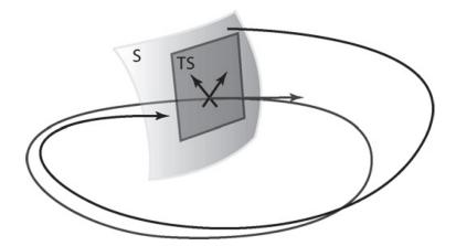
Figure 2.3: Poincaré surface S and linearization TS with periodic orbit  $\gamma$  (grey) and another solution converging to the orbit (black). Illustration © 2008 Elsevier. Reproduced, with permission, from Annual Reviews in Control, vol. 32, no. 2, A. Shiriaev, L. Freidovich, and I. Manchester, "Can we make a robot ballerina perform a pirouette? Orbital stabilization of periodic motions of underactuated mechanical systems," pp. 200 211, 2008.
