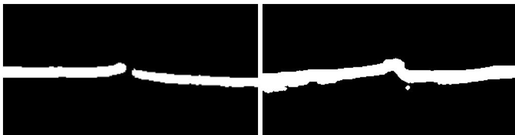
(a) Gap manifested as a gap in the laser line (b) Gap manifested as a bump in the laser line
