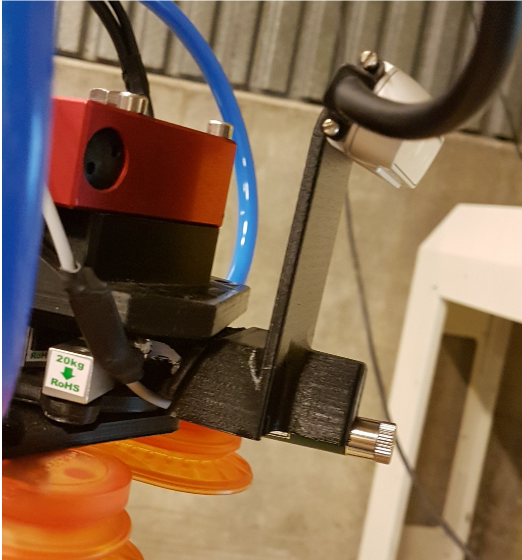
Figure 4.22: Holder mounted on robot, with both laser and camera attached.
