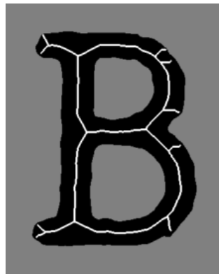
Figure 2.3: Example of skeletonization of an image depicting the letter “B”. Image courtesy of wikipedia
