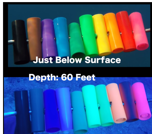
Figure 3.31: The colour loss under water at 20m depth, filmed with a GoPro [19]
