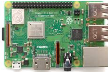
Figure 3.9: Raspberry Pi model 3B+.
