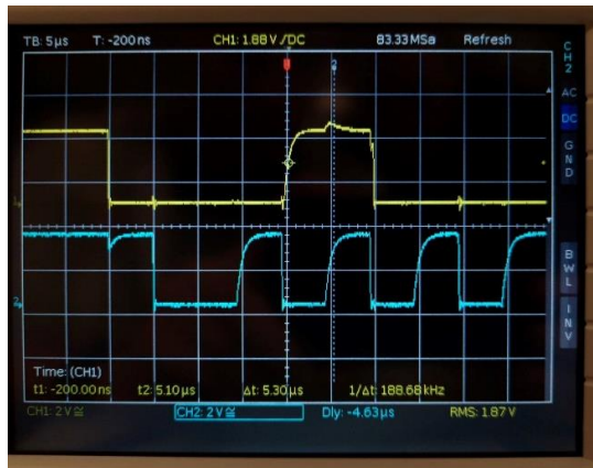
Figure 1 - I2C over 3m cable WITHOUT bus buffer.
