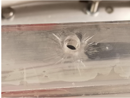
Figure 3.29: Cracks, 4mm plates.
