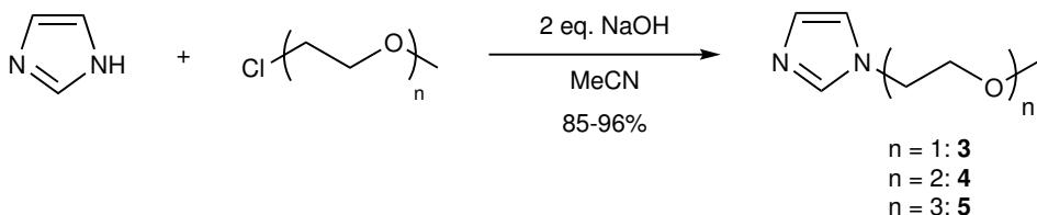
**Scheme 7:** Synthetic procedure of compound **3**, **4** and **5**.
