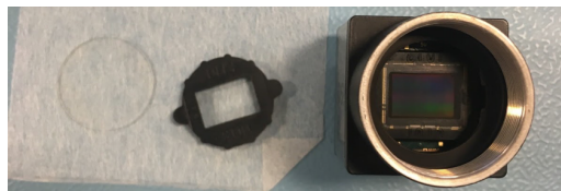
Figure 3.2: Sensor glass and gasket laying on a sheet of cloth, next is the sensor this was taken from.
