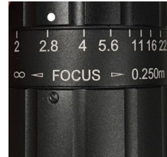
Figure 3.6: The f number was set slightly above 2.8 in what looks like f3
