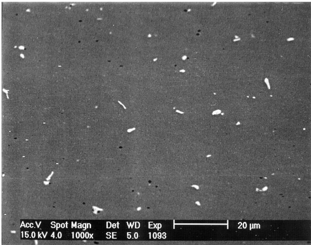
Figure 2.7: SEM micrographs showing the particle structure in the centre of an extruded 6082-profile. The sample is from the material designated P7 in Table 2.2.
