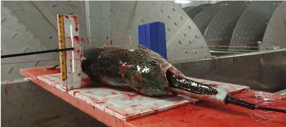
Figure 3.8 Measuring centre temperature and dimensions of salmon
