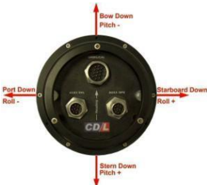
Figure 5: Sign convention for TOGS and MiniRLG strings
