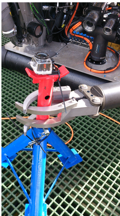
Figure 8.4: Seabed camera mounted on a trestle
