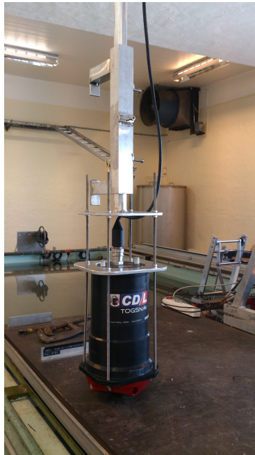
Figure 7.2: TOGSNAV mounted in a welded stand
