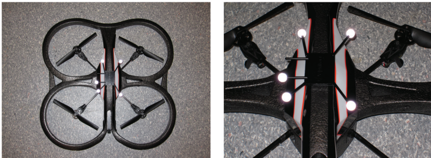
Figure 3.4: The Parrot AR.Drone 2.0 with reflective markers attached to it. The quadcopter is shown to the left, while a close-up of the attached markers is depicted to the right. The collection of markers is placed on top of the quadcopter to exploit the placement of the cameras along the ceiling.
