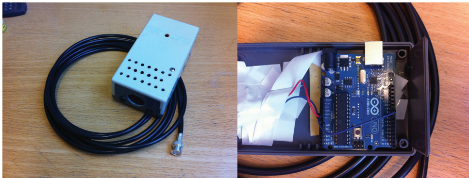
Figure 21: The ECG control unit with BNC interface
