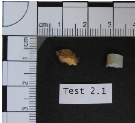
Figure 39: The real(left) and model(right) stone. The model stone was shaped to look match the size of the real stone.
