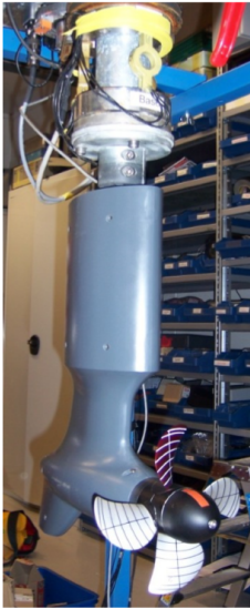
Figure 3-3 Azipull-type thruster body for pulling open propeller used in experiments Kou10. Note the extension of the strut part of the thruster, made to allow variation of the submergence and to ensure that the instrumentation (visible in the top of the picture) came well above the water.
