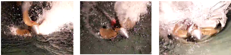
Figure 3-31 Three different propeller position acc. to free surface : propeller is half immersed (middle), propeller hub is 30 mm down to FS (right), propeller hub is 30mm up to FS (left).
