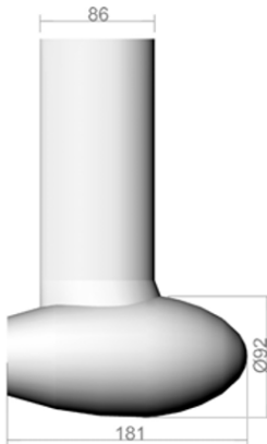
Figure 3-2 Thruster body for ducted propeller used in experiments Kou2006_II.
