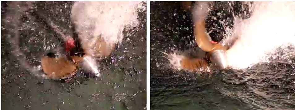
Figure 3-32 Propeller pitch, P/D=15 (left) and P/D=7 (right), which correspond to angle equal to 8 and 18 deg between blade and free surface.
