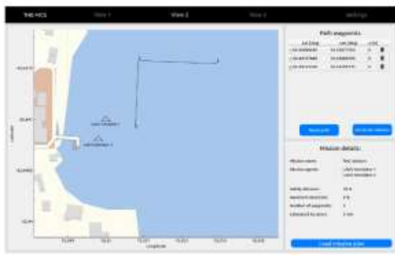
Fig. 4: View 2 of the MCS. Enables defining and reviewing the path for the team and loading the mission plan onto the individual vehicles.
