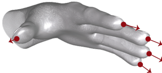
Figure 3.14: Finger tip position and direction vectors provide the position of a finger tip and the general direction in which a finger is pointing [21]
