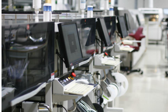
Figure 8.6: The PCBs were soldered in an automated soldering machine
