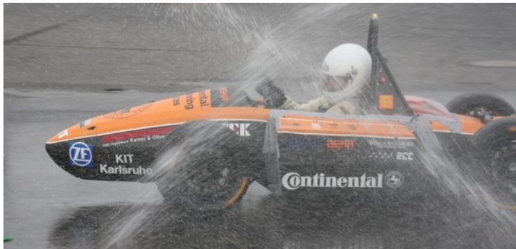
Figure 3.2: Formula Student car during water spray test
