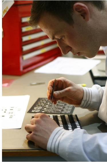
Figure 8.5: Manual placement of components on circuit board
