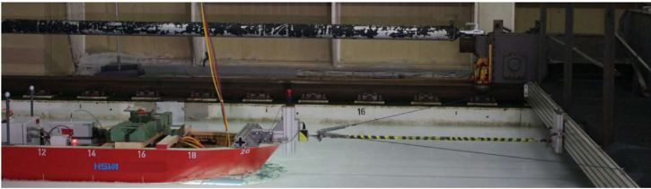
Fig. A11. Execution of towed propulsion test.
