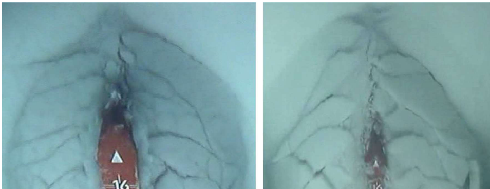
Fig. A5. Breaking pattern of ship model 8 (left) and ship model 9 (right).
