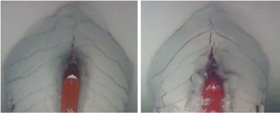
Fig. A1. Breaking pattern of ship model 1 (left) and ship model 2 (right).
