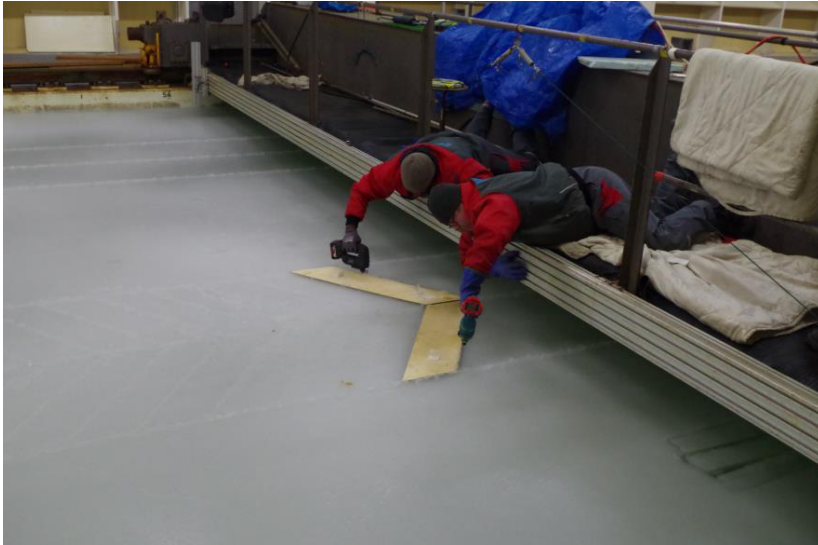
Figure 3: Preparation of the pre-sawn ice sheet
