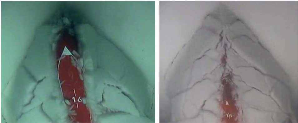
Fig. A6. Breaking pattern of ship model 10 (left) and ship model 11 (right).
