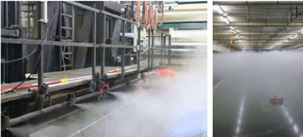
Fig. A9. Water is sprayed into the air of the pre-cooled ice tank at HSVA forming small ice crystals which settle on the water surface.
