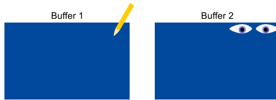
(a) Stage 1 – buffer 1 is draw buffer, buffer 2 display buffer, both buffers contain the same
