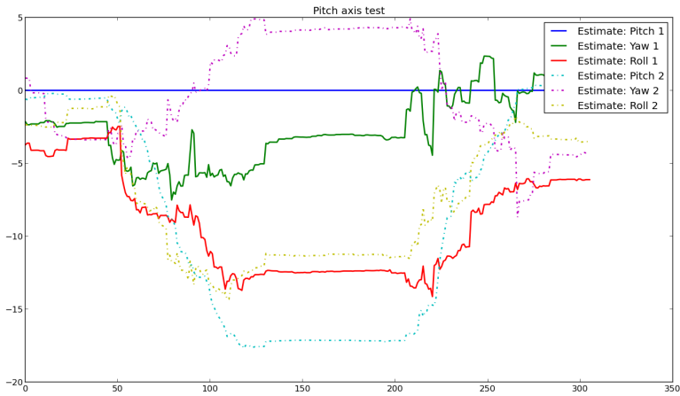
Figure 4.12: The estimated orientations relative to the baseline between the cameras is plotted for each time step.
