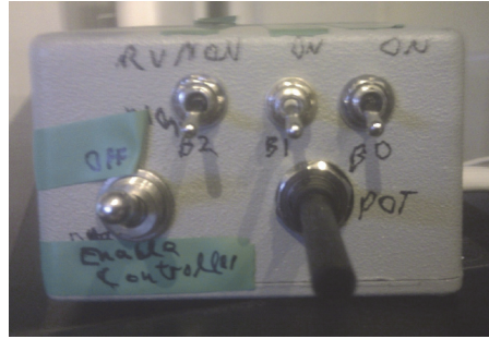
Figure 8: Control box for Piston and Choke
