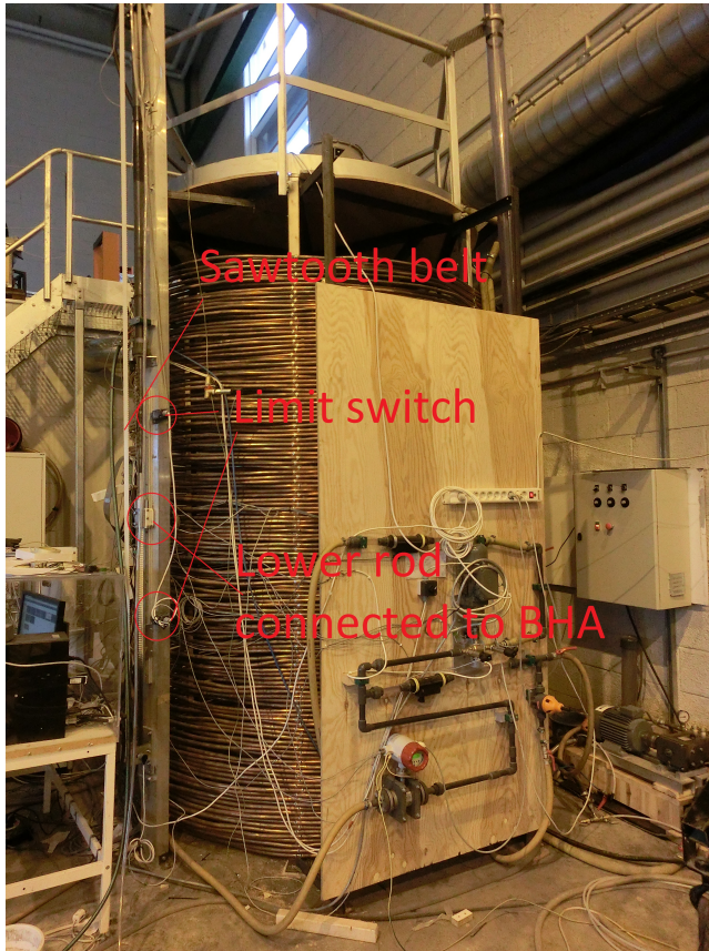
Figur C.4: BHA with limit switches marked.
