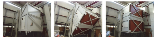
Figure 4. Inclination angles of 0^\circ (vertical pos., left), 45^\circ (middle photo) and 90^\circ (horizontal pos., right) for a tiltable hot box studying impact of air convection on thermal performance of translucent aerogel granule windows [46].
