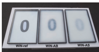
Figure 2. Float glass window panes with (left) air, (middle) large-sized aerogel granulates and (right) small-sized aerogel granulates in the cavities [45].
