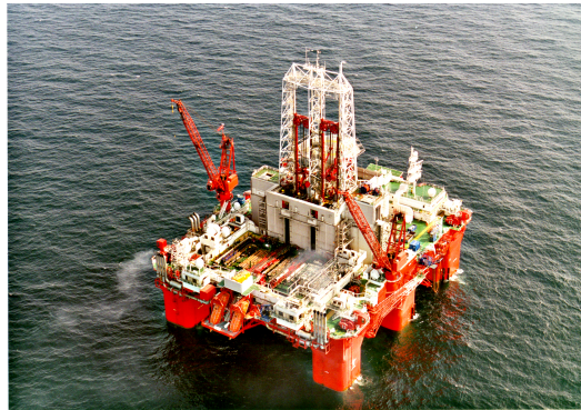
Figure 3.1: Illustration of a semi-submersible. Vessel name: West Venture. Photo: Seadrill.
