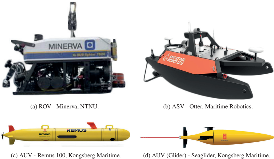
Figure 5.2: The major types of marine robotic platforms: remotely operated vehicles (ROVs), autonomous surface vehicles (ASVs), autonomous underwater vehicles (AUVs), and gliders.
