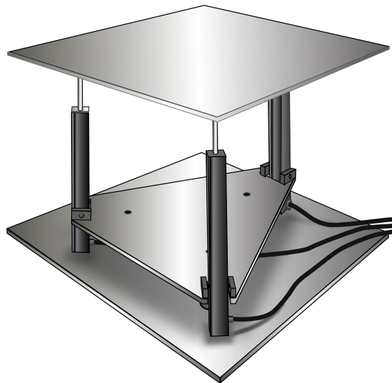
Figure 8.6: The motion platform designed by National Oilwell Varco and built by mechanics at Department of Engineering Cybernetics, NTNU.
