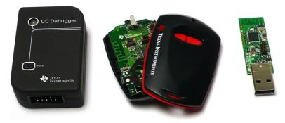
**Figure 10.1:** Texas Instruments' Bluetooth LE evaluation kit. Displayed here: Debugger, KeyFob and USB transceiver dongle. Picture from ti.com.
