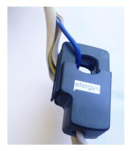
Figure 11.6: Efergy transformer clamp attached to extension cord
