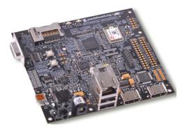
**Figure 12.1:** PandaBoard: 11cm x 10cm includes dual-core 1 GHz ARM Cortex A9, Ethernet, USB, 1GB RAM, SD-card slot, 1080p HDMI out, runs OS from SD-card.
