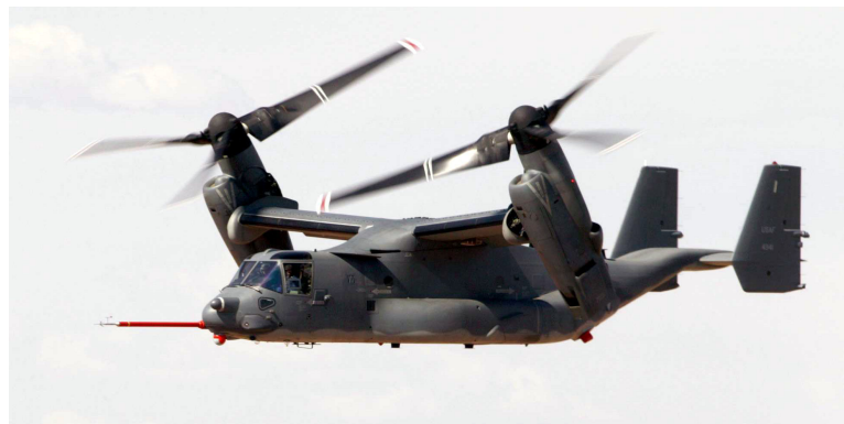
Figure 1.4: Tilt rotor airplane - The tilt rotor airplane has the possibility of rotating its propeller 90 degrees [9].
