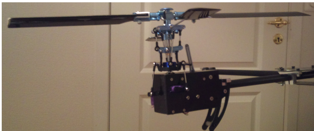
Figure 5.3: Rotor system (450-size) - prototype - The rotor system, made of 3mm plexiglas plates with all the parts assembled
