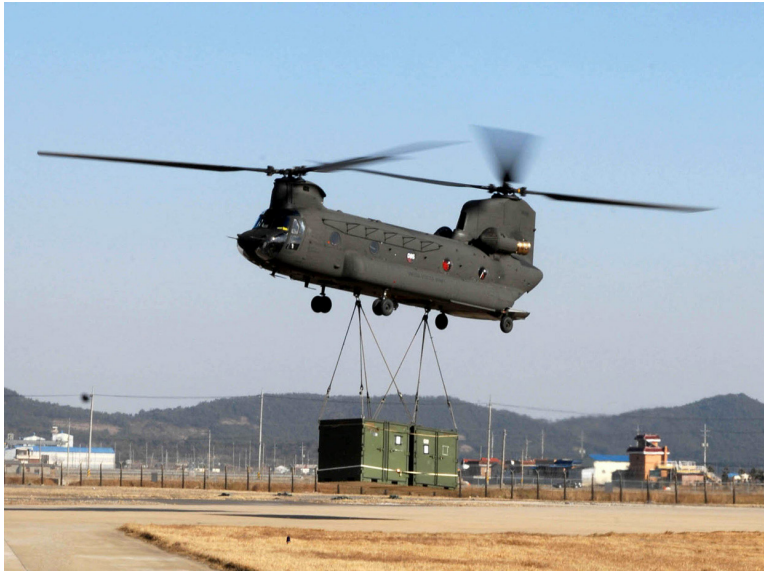
Figure 1.5: Chinook helicopter - The Chinook helicopter has two rotor blades, which rotates the opposite way of each other to counteract yaw movements [18].
