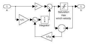
Figure 4.2: Simulink diagram of the PI regulator with anti windup
