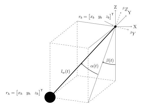
Figure 2.3: Spherical pendulum notation
