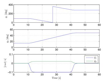
Figure 6.1: Plot of the test signal used for slew  $q_1$  and boom motion  $q_2$
