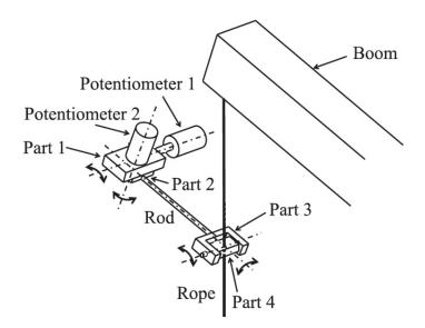
Figure 7.2: Sway measurement of whipline by use of potensiometers [28]
