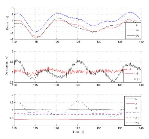
Figure 3.2: Detail view of Kalman filter with two different parameter estimation algorithm as input
