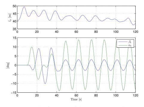
Figure 6.4: Plot of scenario 2 of the rotary crane simulation
