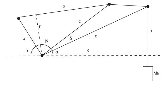
Figure 2.5: Schematic view of the crane geometry
