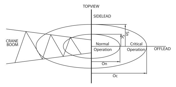
Figure 7.1: Hook position relative to crane boomtip [19]
