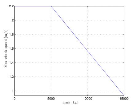
Figure 4.3: Speed profile of 1 fall configuration hoist winch
