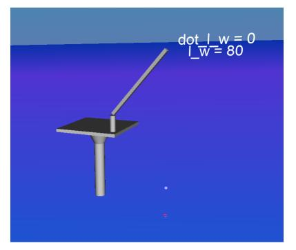
Figure 5.2: Visualisation of rotary crane with spherical pendulum
