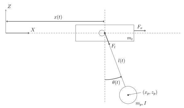
Figure 2.1: Sketch of trolley with pendant load in wire
