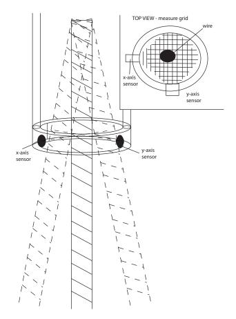
Figure 7.3: Sketch of sensor for measurement of off lead/side lead angle for whip line
