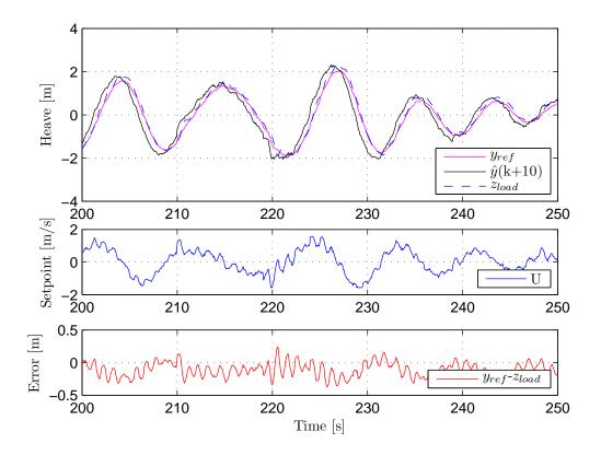
Figure 6.16: Simulation with Kalman predicted set point from camera measurement, 10ton hook load, 1.57m/s max velocity
