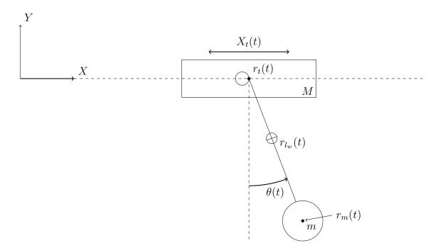
Figure B.1: Sketch of trolley with pendant load in wire
