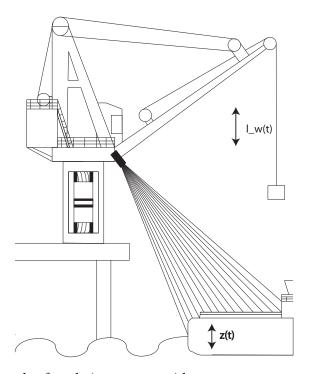
Figure 3.1: Sketch of real-time stereo video camera measurement system
