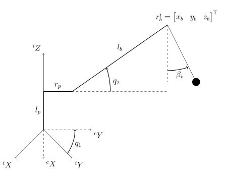
Figure 2.4: Crane-fixed coordinate system c and swing angle notation
