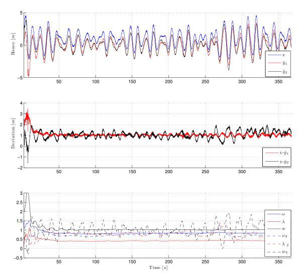
Figure E.1: Comparison between two parameter estimation algorithms as input to the Kalman filter
