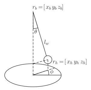
Figure C.1: Sketch of spherical pendulum
