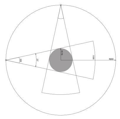
Figure 7.4: Suggestion of Ultrasonic sensor installation
