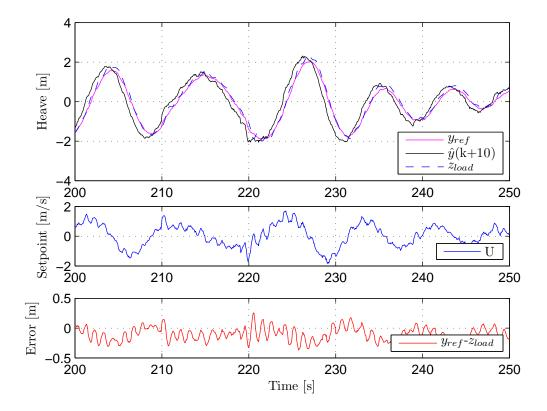
Figure 6.15: Simulation with Kalman predicted set point from camera measurement, 5t hook load, 2.2m/s max velocity
