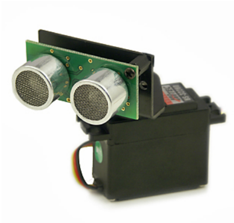
Figure 5.10: Range sensor mounted on a servo.
