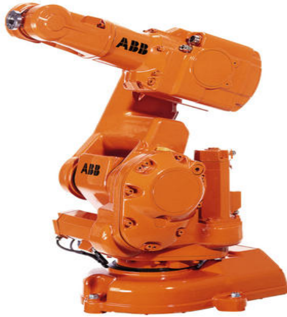
Figure 7.1: ABB IRB140
