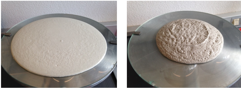
Figure 2 - Spread of mortar (Series 2) 30 min after mixing; left: reference; right: kaolinite.
