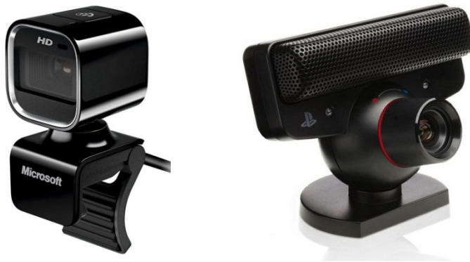
Figure 4-6: Cameras used, Microsoft LifeCam HD-6000 and PS3 eye
