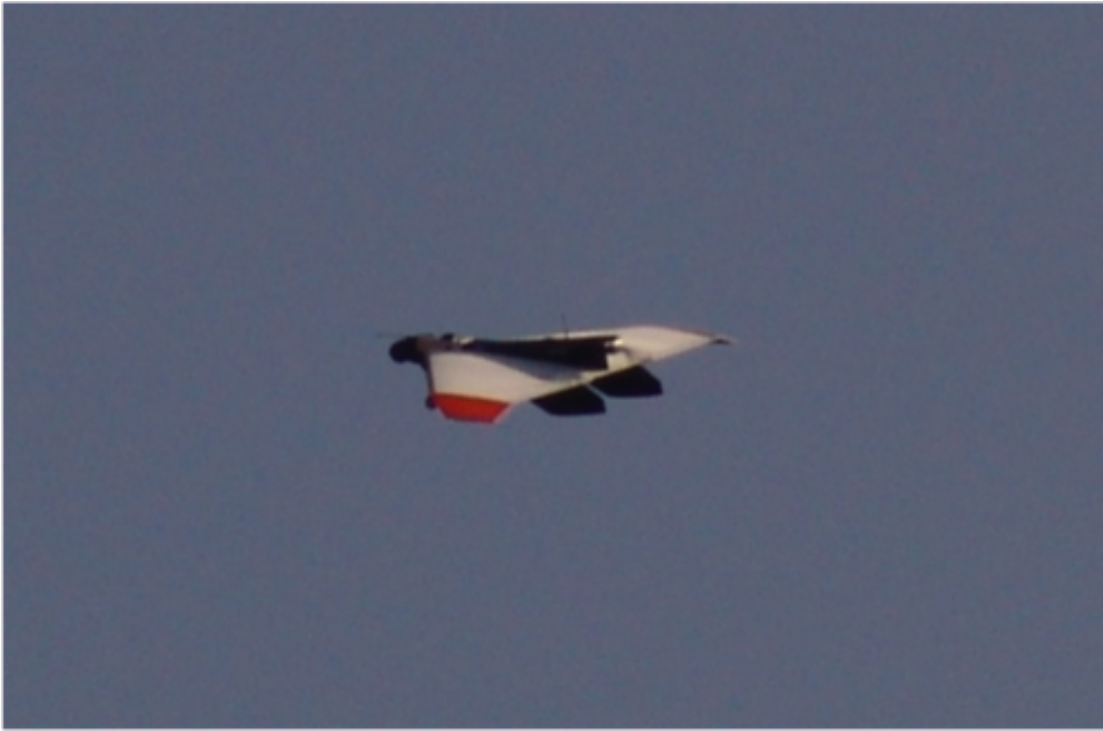
Figure 1.1: Illustration of the Odin Recce D6 delta-wing aircraft (from www.odin.aero )
