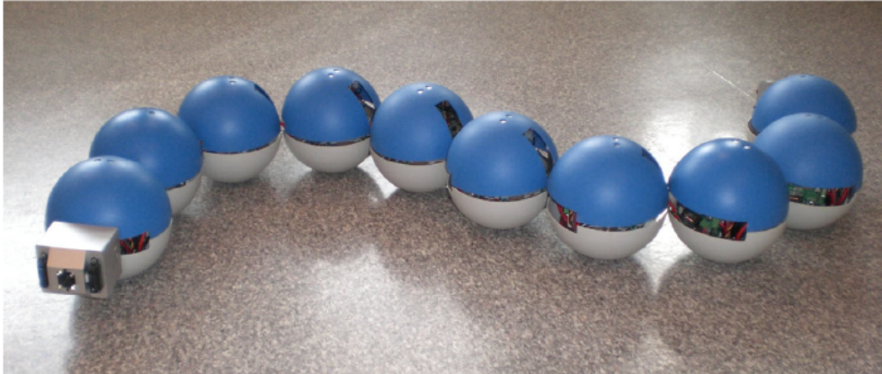
Figure 1.1: The snake robot Kulko developed at NTNU for locomotion in unstructured environments.
