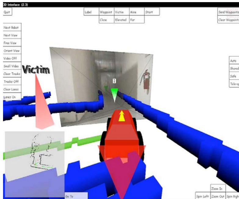
Figure 3.2: Augmented virtuality system with integrated 3D map and third person view. Picture taken from [3].
