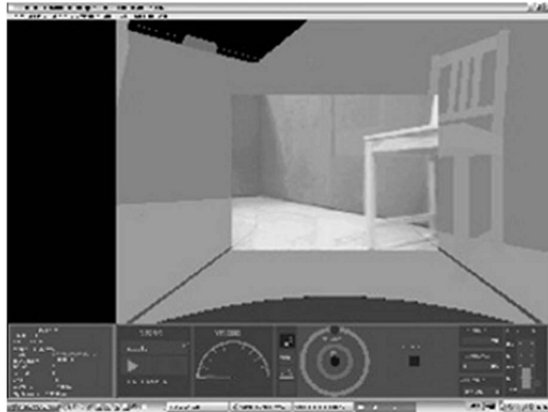
Figure 3.3: Augmented virtuality system to dispel the keyhole effect. Picture taken from [17].
