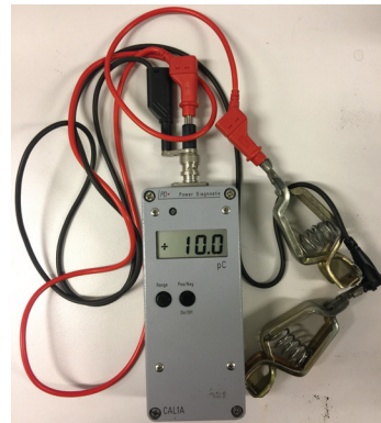
Figure F.4: Impulse injector used for calibration.
