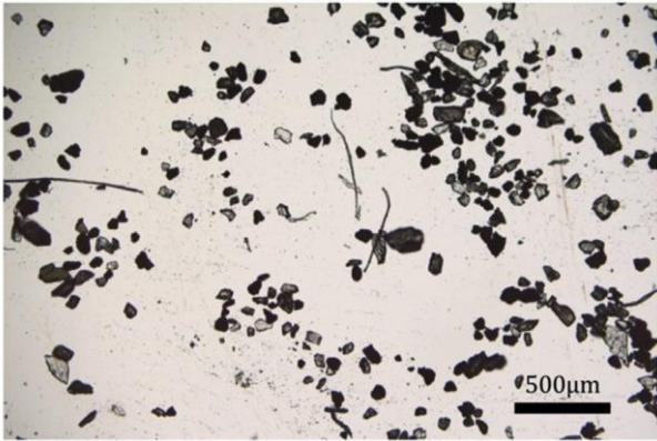
Fig. 14. Wear particles from sawn concrete surface B75. (Fibres came from filtration paper). and varies within the central band. Furthermore, mild abrasion is concentrated in the same spots as severe abrasion but with a lower rate. In the case of sawn surfaces, the abrasion is localized in the bond zone between mortar and coarse aggregates (Fig. 8.). This can be related either to the mechanical properties in the interfacial transition zone (ITZ) or to uneven stress distribution due to the different phases of concrete in the concrete-ice contact zone resulting in stress concentration. So, the ITZ seems to be a weak point for the onset of wear, and it would be interesting to make a closer study of the evolution of the abrasion there, perhaps with the 3D optical microscope.
