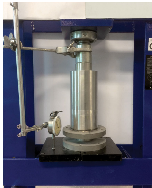
Fig. 6 Setup for the compaction of the gouge material
