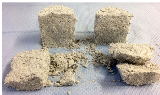
Fig. 11 Test sample 2-8 split after testing to check quality of water addition. In the case of dry zones, they were easy to detect
