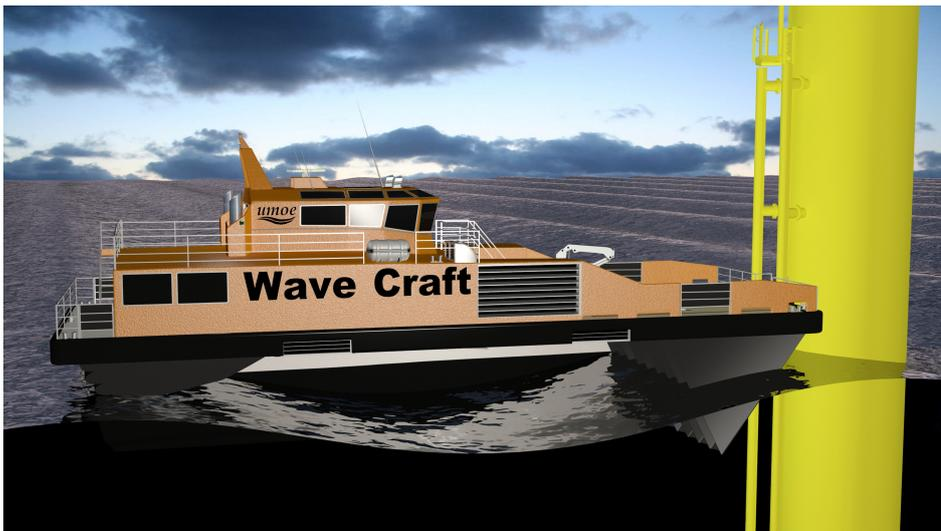
Figure 7.8: The Wave Craft at zero speed in control mode next to a wind turbine. The vessel bow is the control point. A video simulating the motion damping can be found in the DVD enclosure. See "Wave Craft at turbine.wmv"
