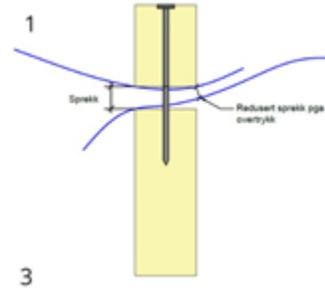
Shrinkage of the batten and the stud reduces the clamping effect leaving a air gap between the batten and the stud.
