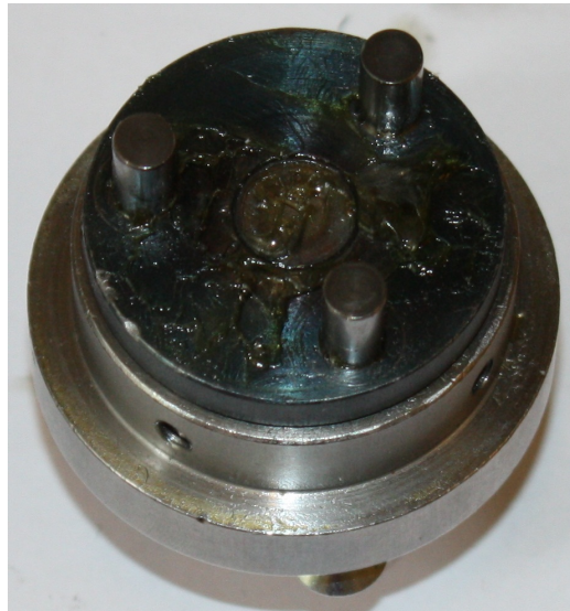
Figure 5.1: Image showing the broken third stage of the planetary gearbox.
