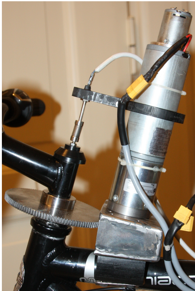
Figure 5.3: Image showing the new steer gear and transmission assembly
