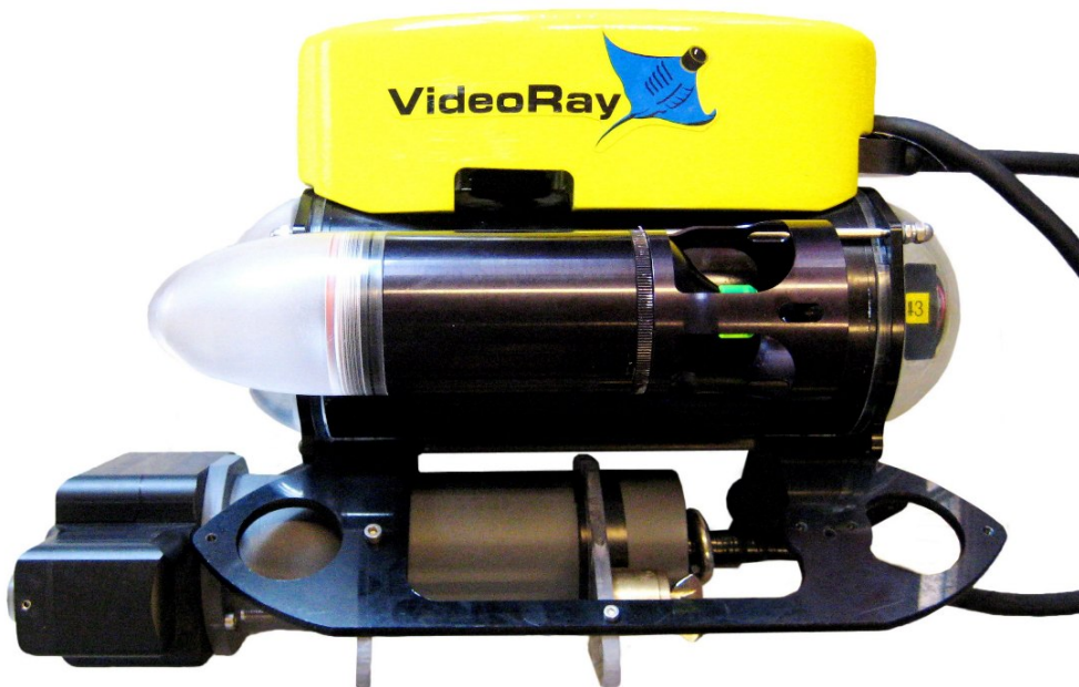
Figure 6.2: Laser module attached to ROV
