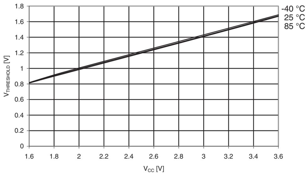
**Figure 35-31.** Reset Input Threshold Voltage vs.  $V_{CC}$
