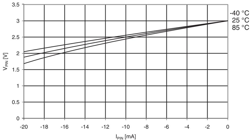
**Figure 35-23.** I/O Pin Output Voltage vs. Source Current
