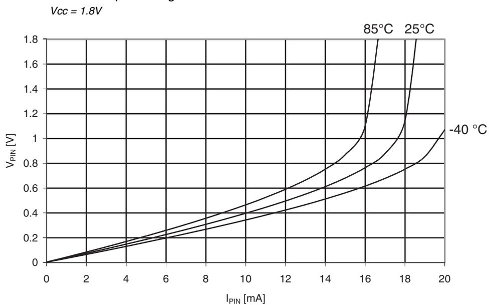
**Figure 35-25.** I/O Pin Output Voltage vs. Sink Current
