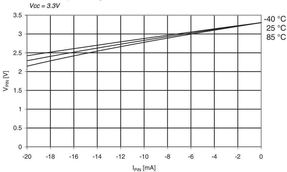
**Figure 35-24.** I/O Pin Output Voltage vs. Sink Current
