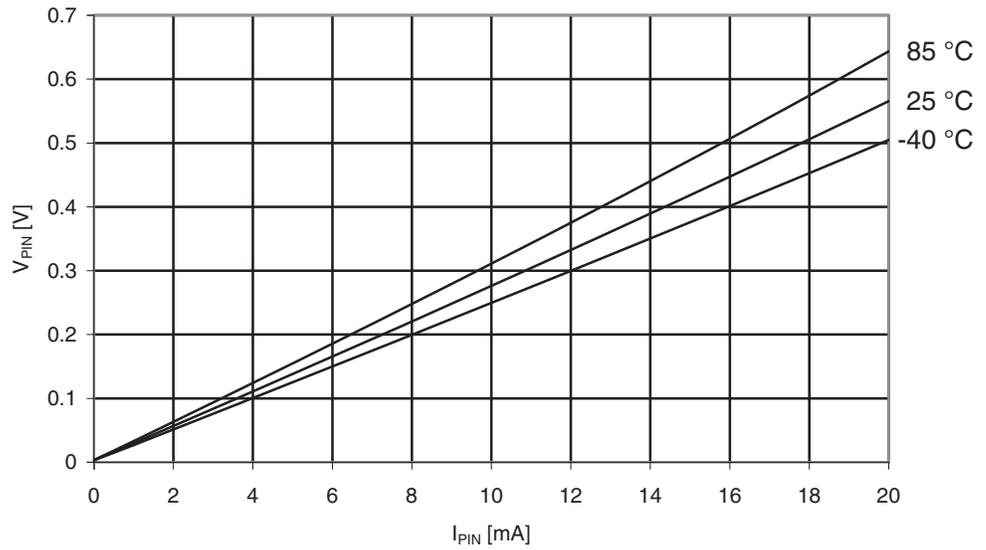
**Figure 35-26.** I/O Pin Output Voltage vs. Sink Current
