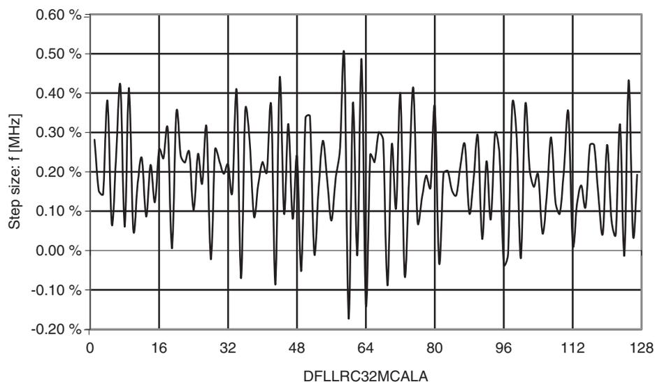
**Figure 35-38.** Internal 32 MHz Oscillator CALB Calibration Step Size
