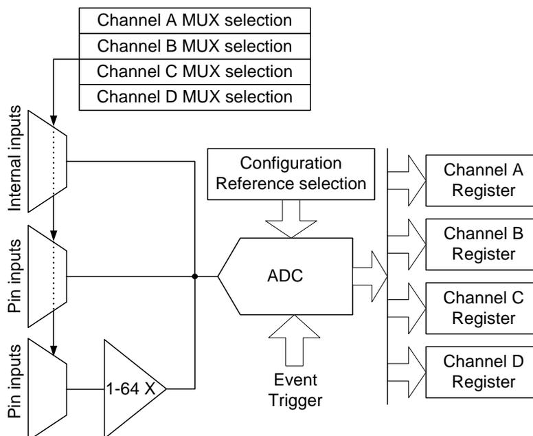
Each ADC has four MUX selection registers with a corresponding result register. This means that four channels can be sampled within 1.5  $\mu\text{s}$  without any intervention by the application other than starting the conversion. The results will be available in the result registers.
