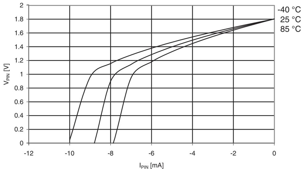
**Figure 35-22.** I/O Pin Output Voltage vs. Source Current
