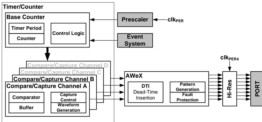
The Hi-Resolution Extension can be enabled to increase the waveform generation resolution by 2 bits (4x). This is available for all Timer/Counters. See ["Hi-Res - High Resolution Extension"](#) on page 34 for more details.
