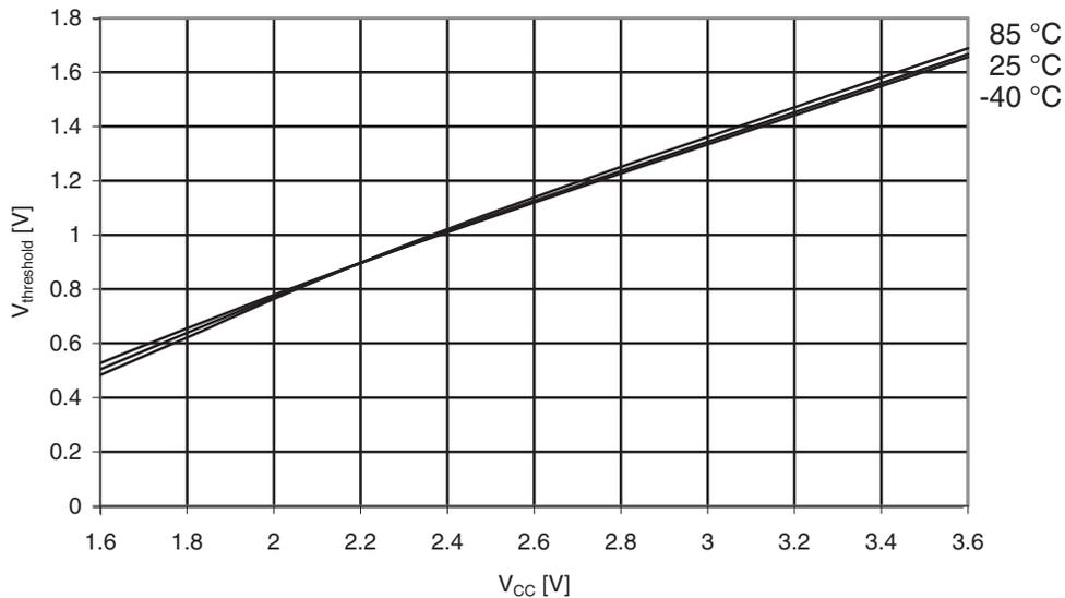
**Figure 35-29.** I/O Pin Input Hysteresis vs.  $V_{CC}$
