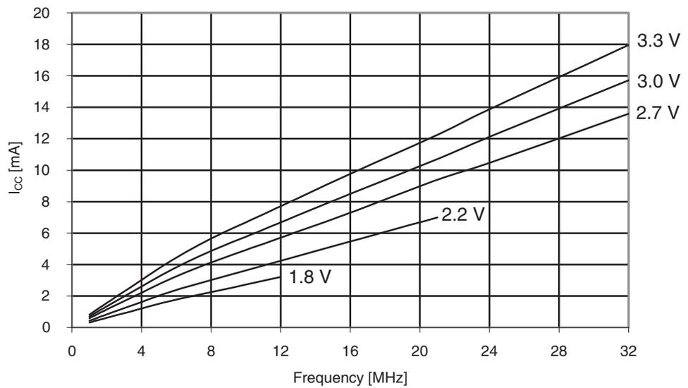
**Figure 35-3.** Active Supply Current vs. Vcc
