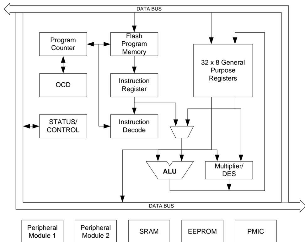
The AVR uses a Harvard architecture - with separate memories and buses for program and data. Instructions in the program memory are executed with a single level pipeline. While one instruction is being executed, the next instruction is pre-fetched from the program memory.
