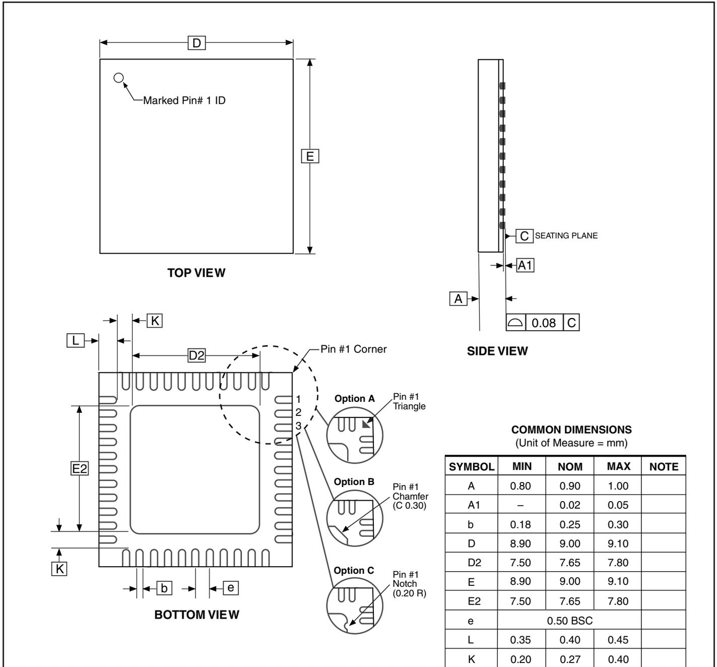
Note: 1. JEDEC Standard MO-220, (SAW Singulation) Fig. 1, VMMD.
