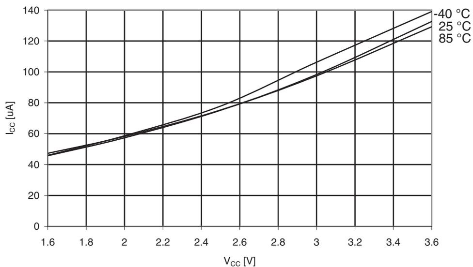
**Figure 35-5.** Active Supply Current vs. V<sub>CC</sub>
