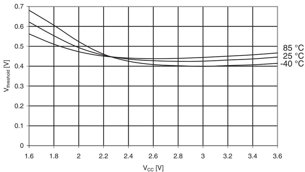
**Figure 35-30.** Reset Input Threshold Voltage vs.  $V_{CC}$
