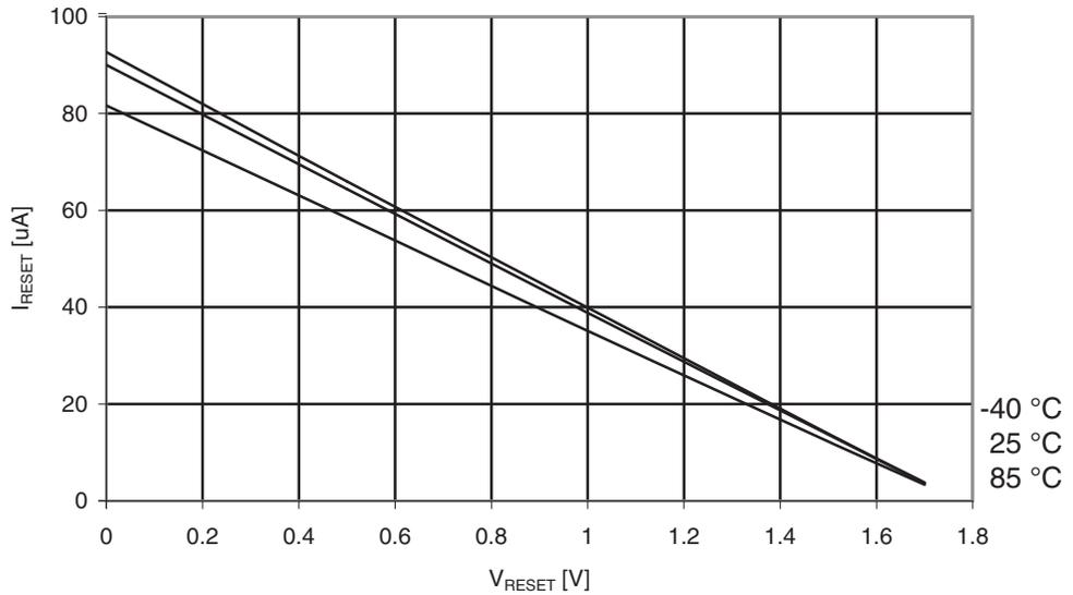
**Figure 35-19.** Reset Pull-up Resistor Current vs. Reset Pin Voltage
