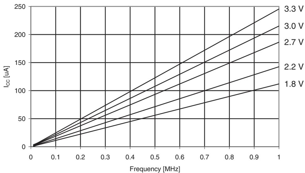
**Figure 35-9.** Idle Supply Current vs. Frequency
