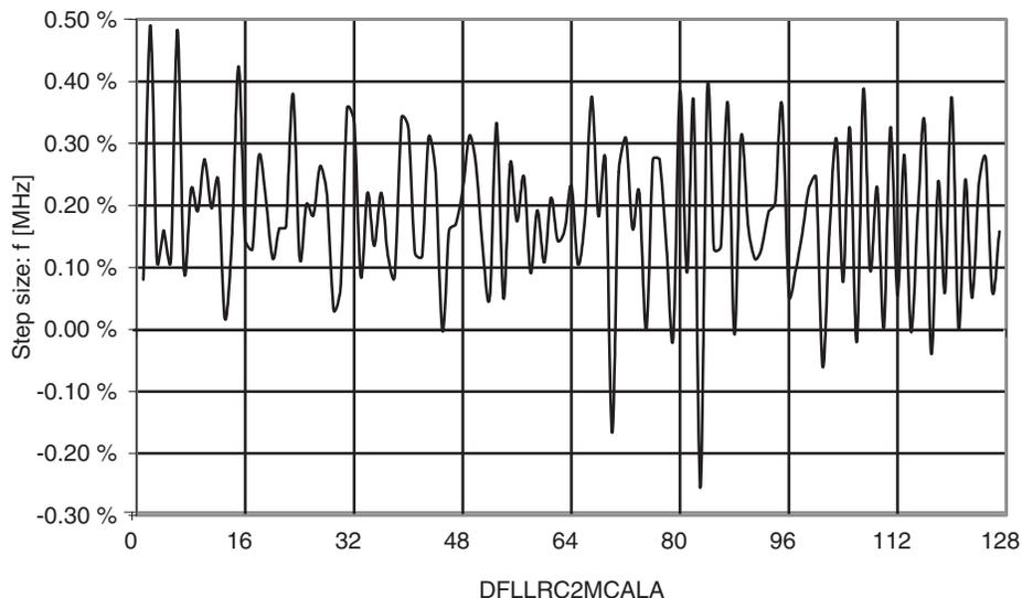
**Figure 35-36.** Internal 2 MHz Oscillator CALB Calibration Step Size
