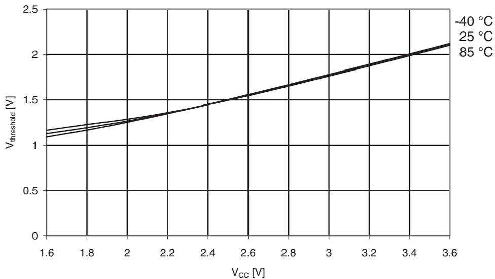
**Figure 35-28.** I/O Pin Input Threshold Voltage vs.  $V_{CC}$
