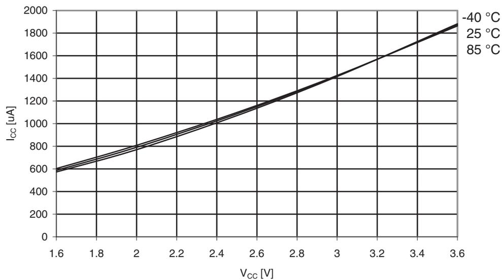
**Figure 35-6.** Active Supply Current vs. V<sub>CC</sub>
