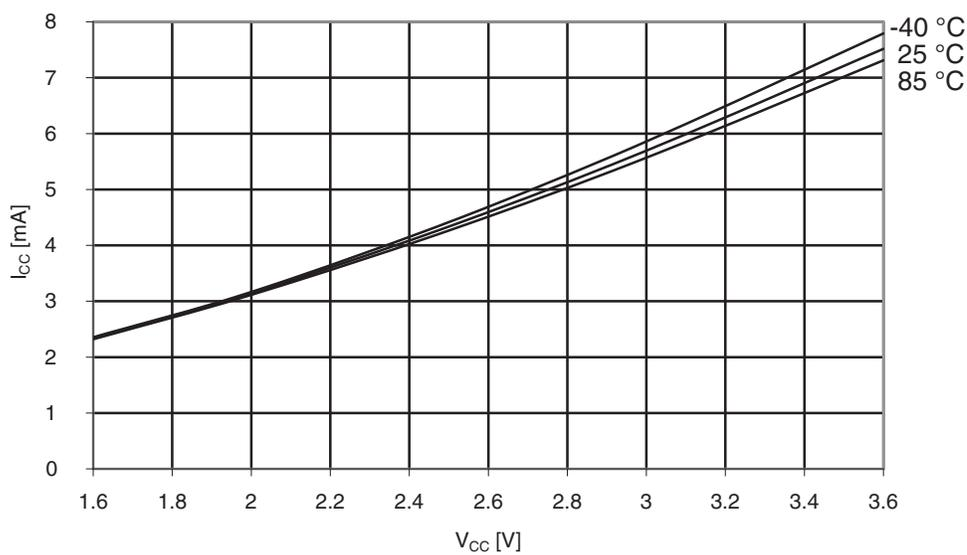
**Figure 35-7.** Active Supply Current vs. V<sub>CC</sub>
