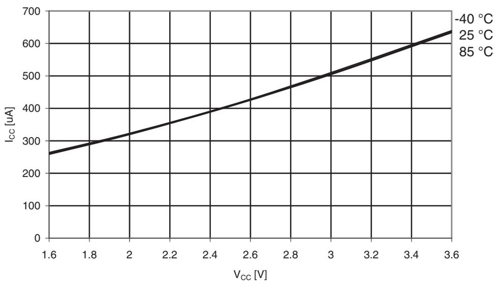
**Figure 35-13. Idle Supply Current vs. Vcc**
