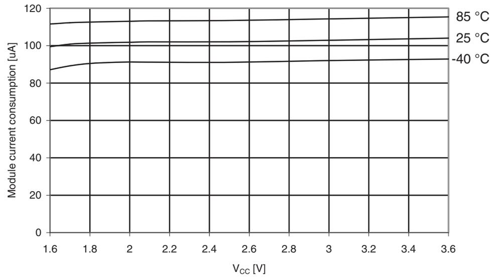
**Figure 35-40.** Power-up current consumption vs. V<sub>CC</sub>
