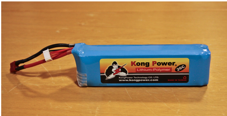
Figure 5.8: Kong Power battery for the NAROM UAV. Power is supplied through the thicker wires while the white connector is used for balancing the battery cells during charge.
