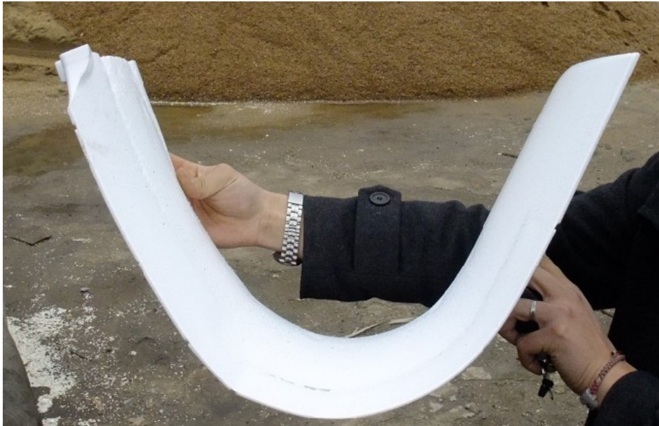
Figure 5.5: The EPO foam is extremely forgivable and can retain its former shape even after heavy strains. This picture displays an actual Skywalker EPO wing section. Photo from the RC group web-page: http://tinyurl.com/6zo6sf5 .
