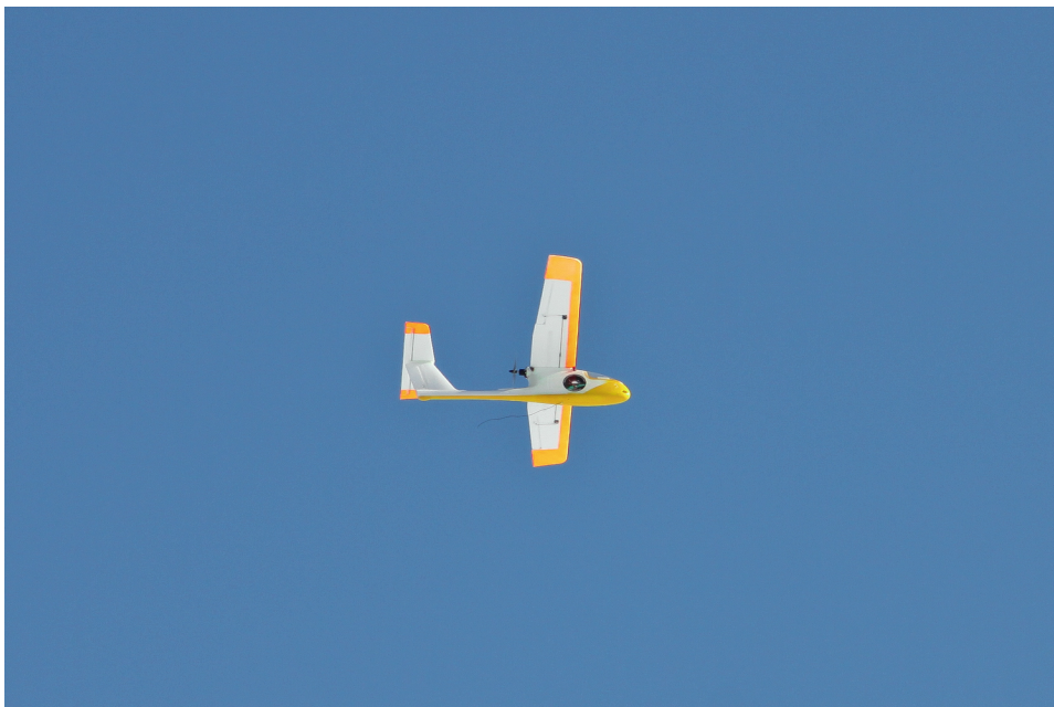
Figure 7.7: The NAROM UAV photographed during its maiden flight. Notice the RC antenna hanging from below the airframe.
