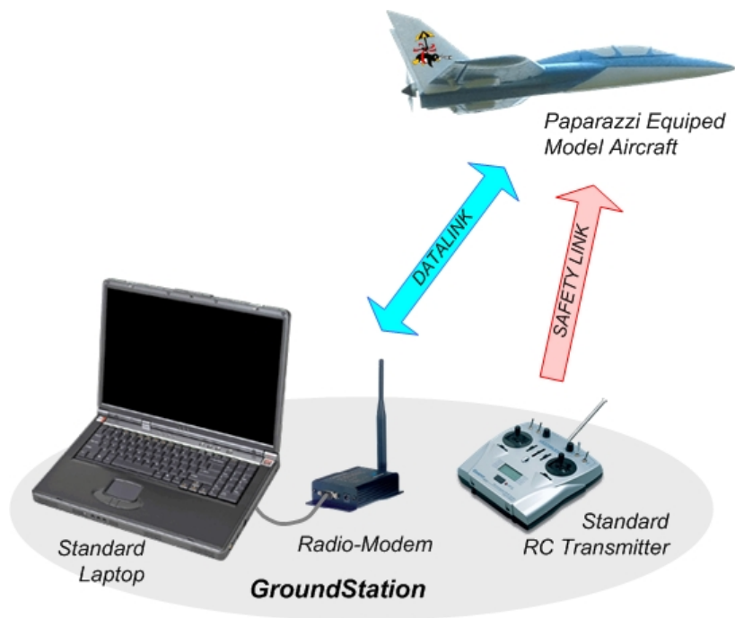
Figure 5.14: Principle drawing of the Paparazzi UAS components. Illustration from the Paparazzi main site, reproduced under the GNU agreement.
