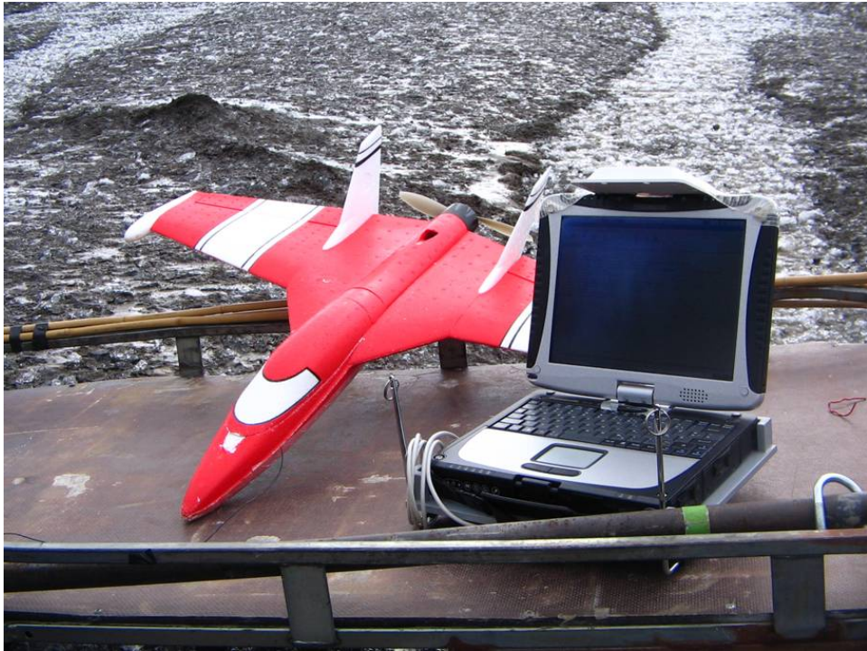
Figure 3.1: The SUMO UAS (Small Unmanned Meteorological Observer) operates as a recoverable radiosonde, and is based on the model airplane "FunJet" by Multiplex. Photo by Marius Jonassen.
