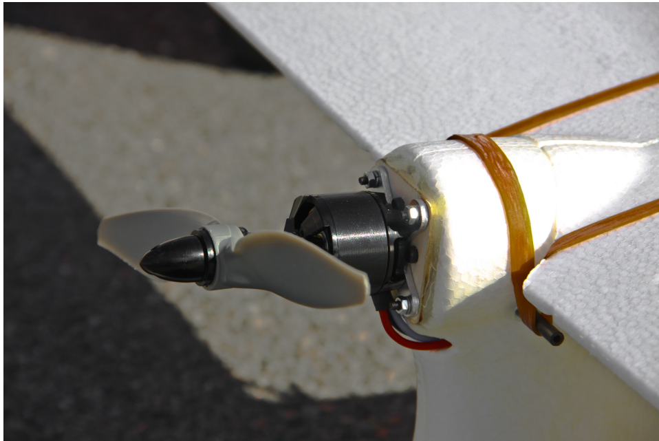
Figure 7.4: Close-up photo of the motor mount. The AX2814 motor is an "outrunner", meaning that the motor spins its outer shell around its windings. Notice the rubber band used for wing attachment.
