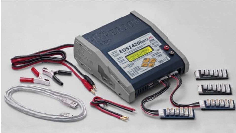
Figure 5.9: Hyperion EOS 1420i NET3 LiPo battery charger. Connection boards for balancing LiPo batteries are shown in the right corner.
