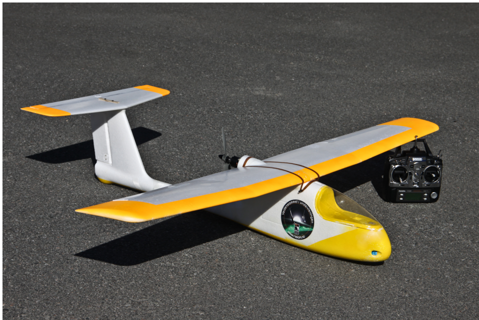
Figure 7.5: The finished NAROM UAV Skywalker EPO airplane. The battery (azure blue) is visible through the ventilation opening in the nose. The Futaba 7CAP RC transmitter is shown in the background.
