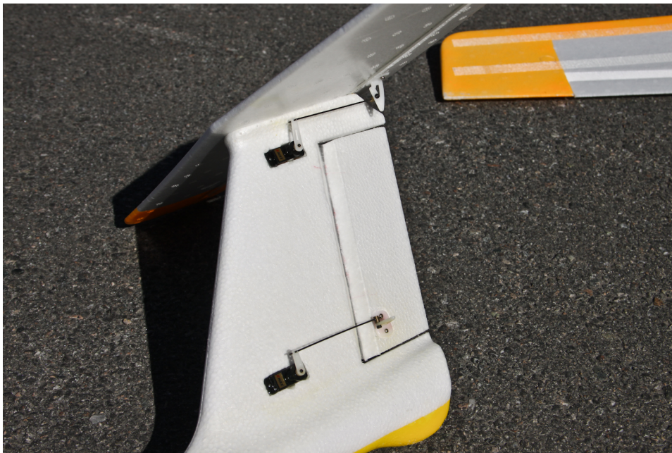
Figure 7.3: Airplane T-tail section. Rudder and elevator servos and links are visible.
