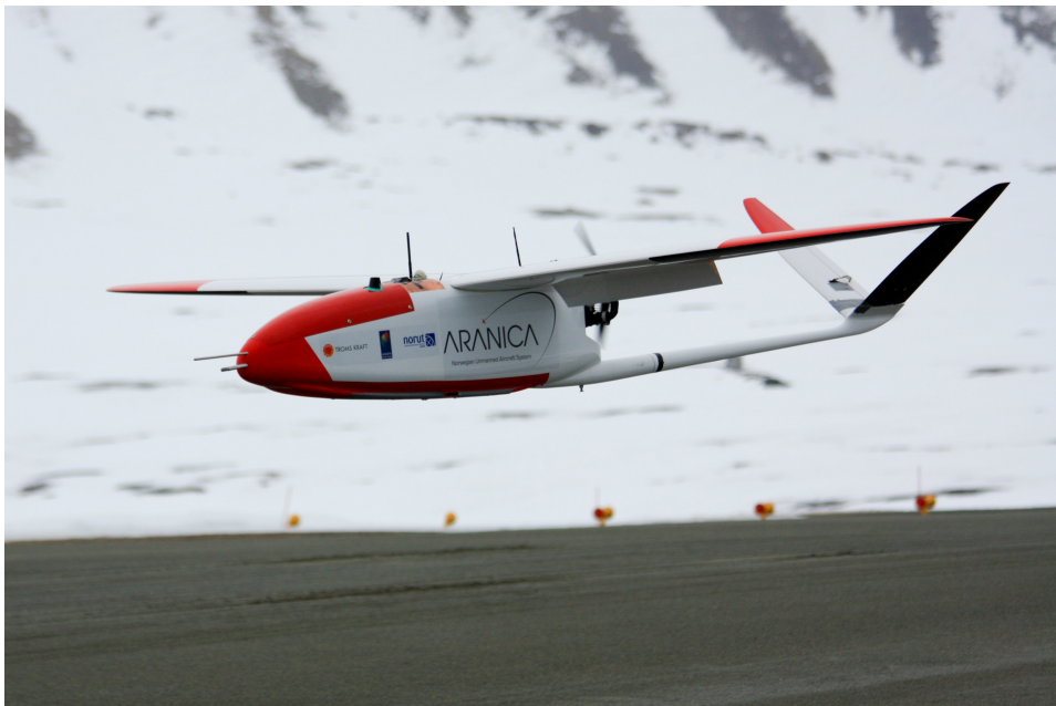
Figure 2.2: Close-up photo of the Cryowing UAV. The wingspan of this UAV is 3.8 m, maximum take of weight is 30 kg, and the maximum range is 500 km/5 hours[26]. Photo by Torbjørn Houge.
