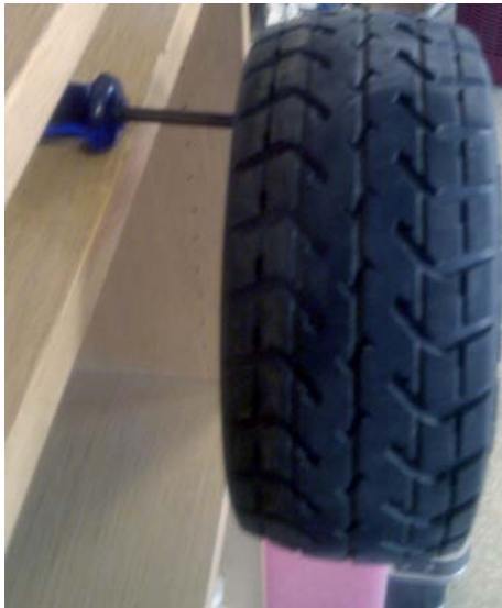
Figure 5.7: Experimental setup for measurement of the wheel moment of inertia.
