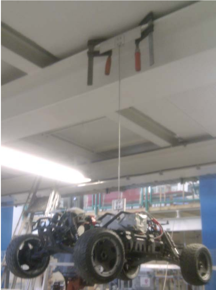
Figure 5.10: Experimental setup for measurement of the moment of inertia around the vehicle z-axis.
