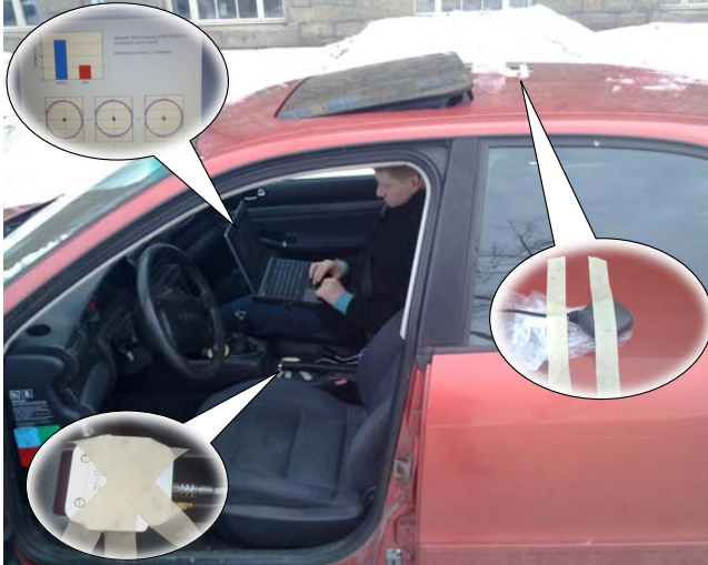
Figure 5.4: Test setup for logging of IMU data.
