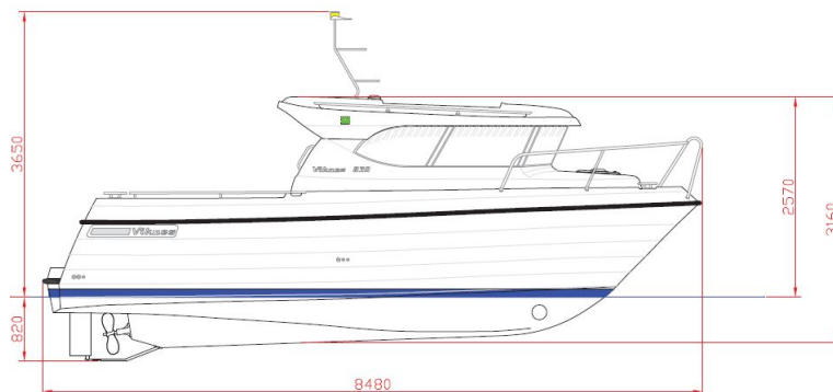
Figure 2.2: The lateral dimensions of the Viknes.
