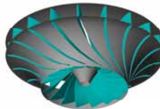
Initial replacement runner (F-100)
