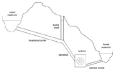
Figure 1 Pump storage plant layout
