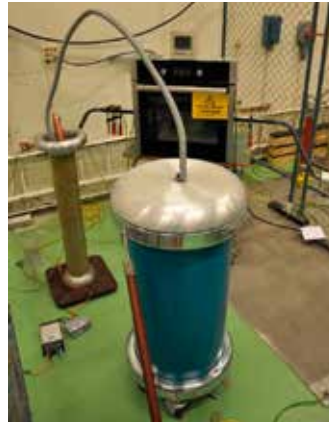
Laboratory test setup for partial discharge (PD) testing at 50 Hz. Transformer in front, connected to a coupling capacitor and the generator winding in back. An oven is surrounding the winding and enables measurements at different temperatures
