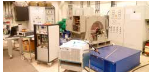
Experimental set-up: 100 kVA, 14 poles salient pole synchronous generator
