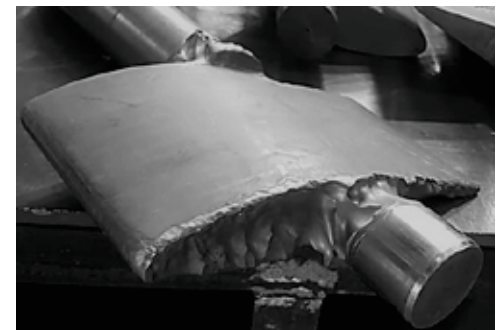
Erosion at Guide Vane's facing ends and facing plates at Bhilangana-III HEP
