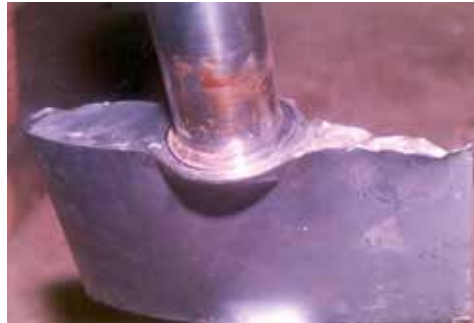
Sand erosion on a guide vane blade
