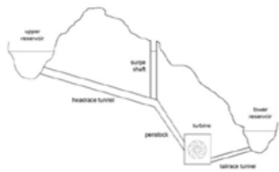
Figure 1 Pump storage plant layout
