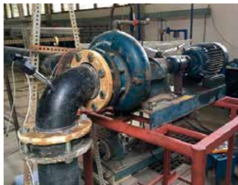
Part of the test rig at UDSM used for model validation, with the pump used as turbine installed
