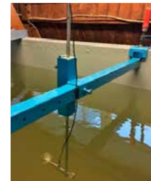
From project thesis: Propeller current measurements in the free surface loop at the Water power Laboratory at NTNU.
