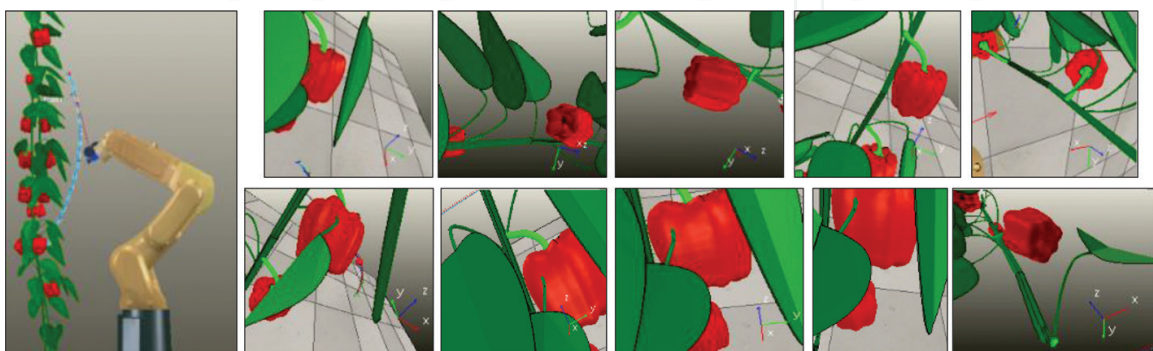
Figure 21. Three dimensional scanning experiments ( x - y - z space) for finding the maximum fruit visibility. Camera was set to rotate around the fruit and plant until it finds the best angle of attack.
