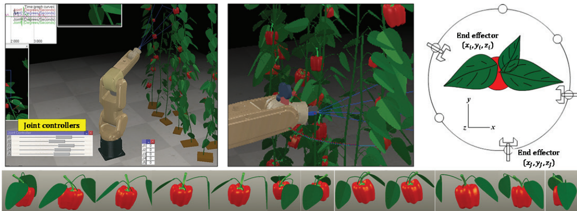
Figure 20. Two dimensional scanning experiment ( x - y , x - z , and y - z planes) for finding the maximum fruit visibility. Camera was set to move at 30 degrees increments around the fruit and plant model.
