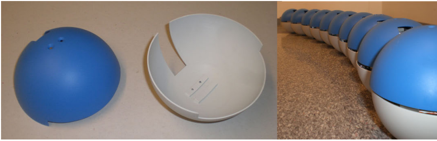
Figure 11.2: Left: The upper and lower hemispherical shell of a joint module. Right: The smooth gliding surface along the snake robot.
