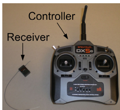
Figure 11.12: The remote controller and the receiver used for demonstrating the snake robot.
