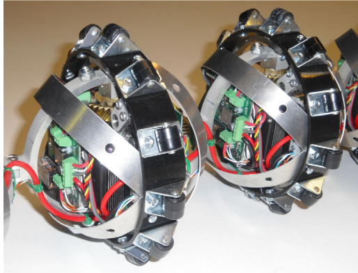
Figure 3.6: A ring with 12 plastic wheels encloses each joint module in order to give the robot anisotropic ground friction properties.
