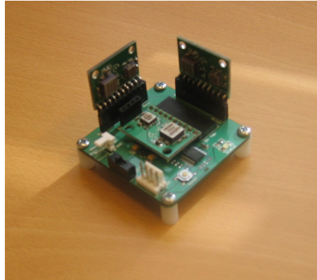
Figure 3.11: IMU from Spark Fun Electronics with 6 degrees of freedom. Picture from [Loftum, 2006]
