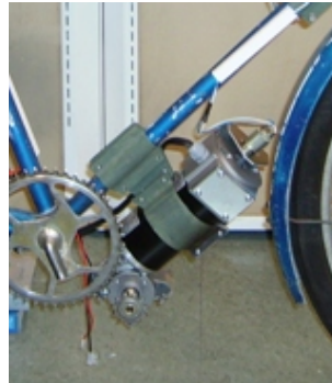
Figure 3.7: The propulsion motor; a Lenze Worm Geared motor. Picture from [Sølvberg, 2007]
